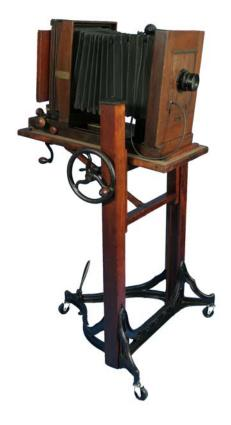
This is a Kodak No. 10A Century Studio Camera (8" × 10" format size) mounted on a Kodak No. 1A Semi-Centennial Stand, manufactured by the Folmer & Schwing Department of Eastman Kodak Company in late 1925 or early 1926.
