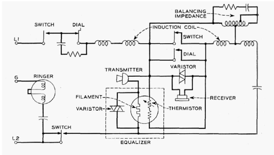
The astute reader may wonder about the apparent short-circuit across part of one winding of the induction coil (transmission transformer) near the label "balancing impedance" (which would better be pointed up to the nearby resistor and capacitor).
