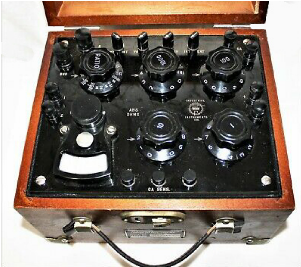
Figure 3. Leeds & Northrup portable Wheatstone bridge
