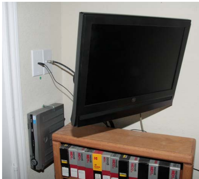
Figure 2. Motorola VIP1200 STB and Westinghouse TV set (our installation)
