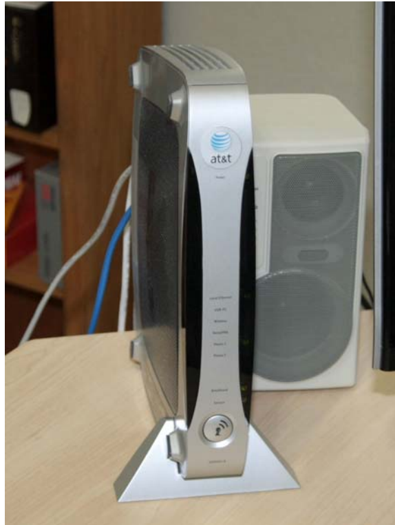
Figure 1. Residential gateway (RG)—2Wire 3800HGV-B (our installation)
