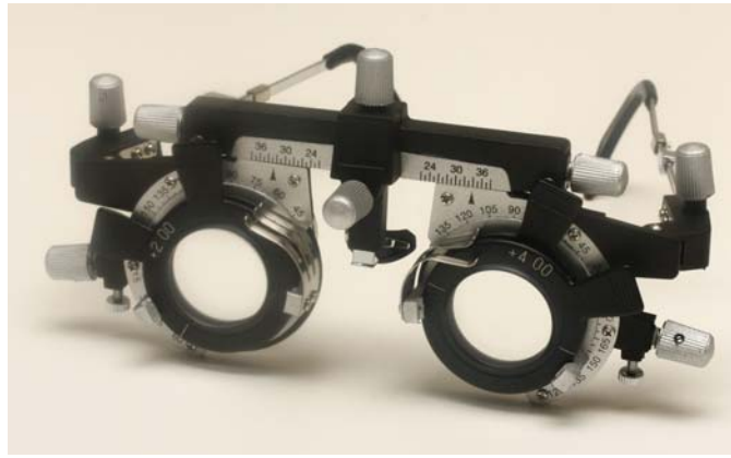
Figure 8. Modern trial frame with modern trial lenses
