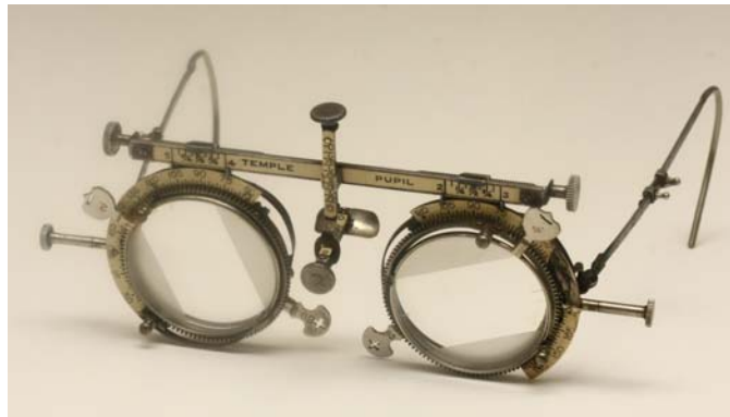
Figure 9. Antique trial frame with traditional trial lenses
