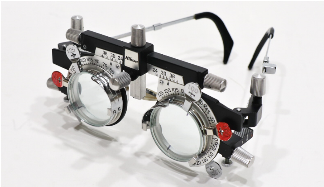
Figure 3. Trial frame with lenses in positions 1, 2, and 3
