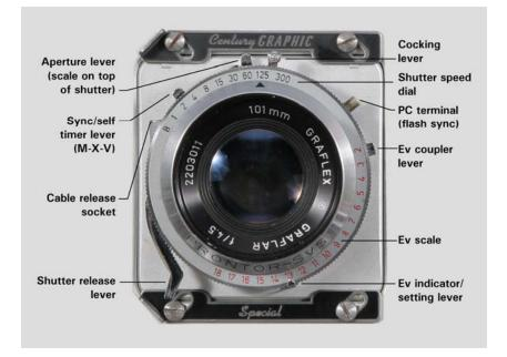
The Ev coupler lever determines whether or not, as the shutter speed dial is turned, the aperture setting also changes to maintain the Ev shown (or set) by the Ev indicator. The coupler is disengaged if the photographer wishes to set shutter speed and aperture independently and just be able to see the
