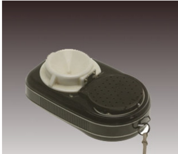
Figure 7. Weston Invercone incident light diffuser (original type)
