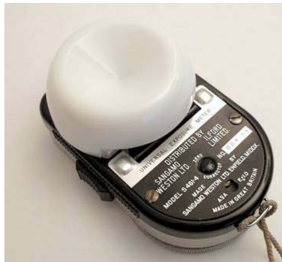
Figure 8. Weston Master IV meter with Invercone (newer type)
