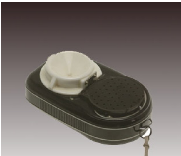
Figure 7. Weston Invercone incident light diffuser (original type)
