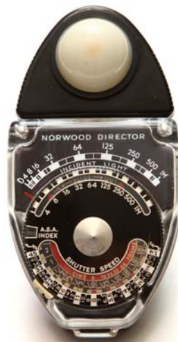
Figure 5. Norwood Director exposure meter, Model B
