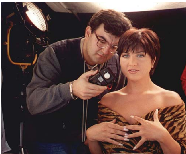
Figure 2. Incident light exposure measurement
