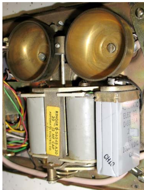
Figure 10. Automatic Electric Company frequency selective ringer
