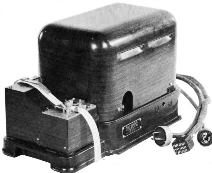
Figure 9. Typical Model 14 receiving transmitter distributor
