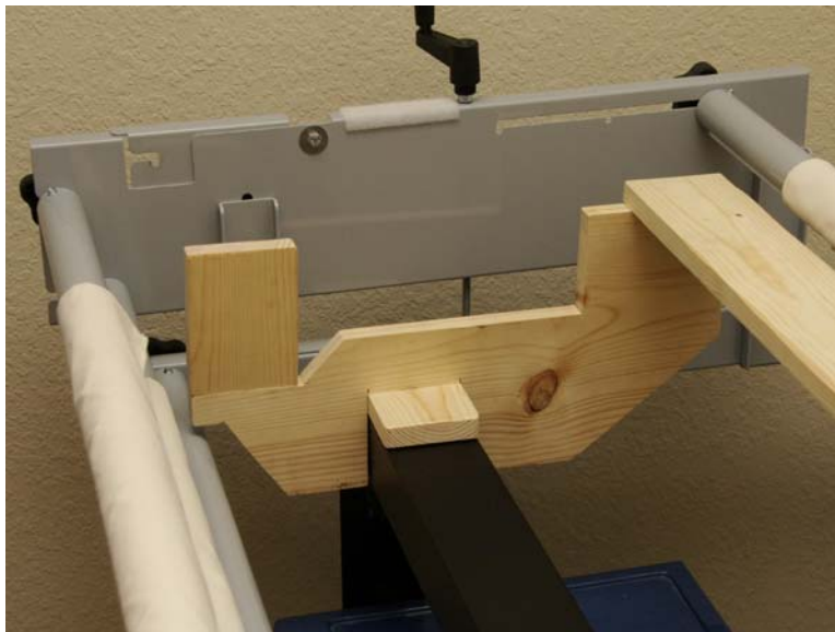
Figure 21. Shelf in position for pinning sandwich
