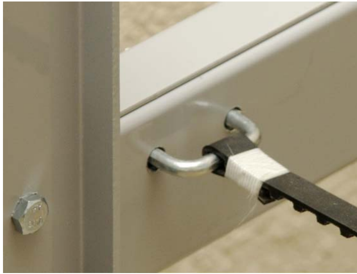
Figure 9. X-direction toothed belt attachment
