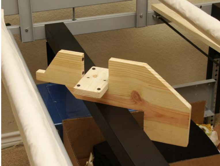
Figure 14. Pinning shelf support
