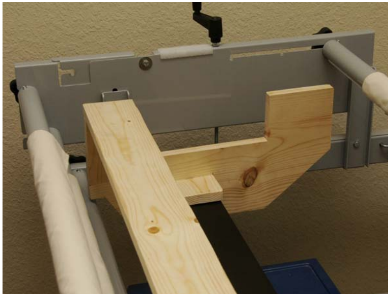
Figure 19. Shelf in position for pinning the back
