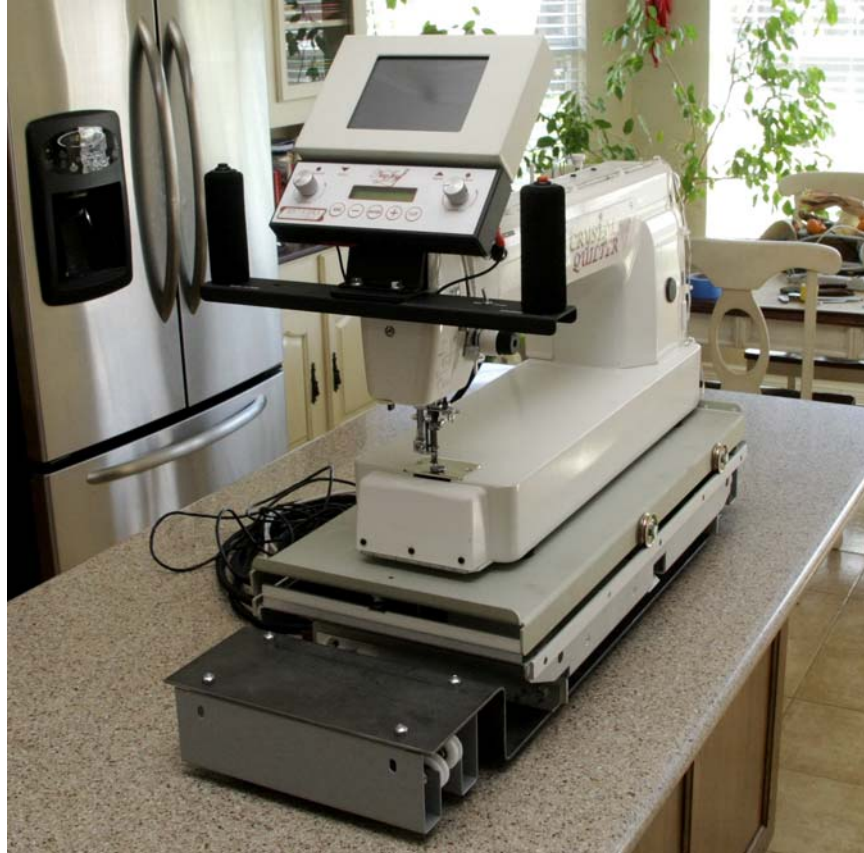
Figure 6. Crystal Quilter head on adapted PCQ carriage
