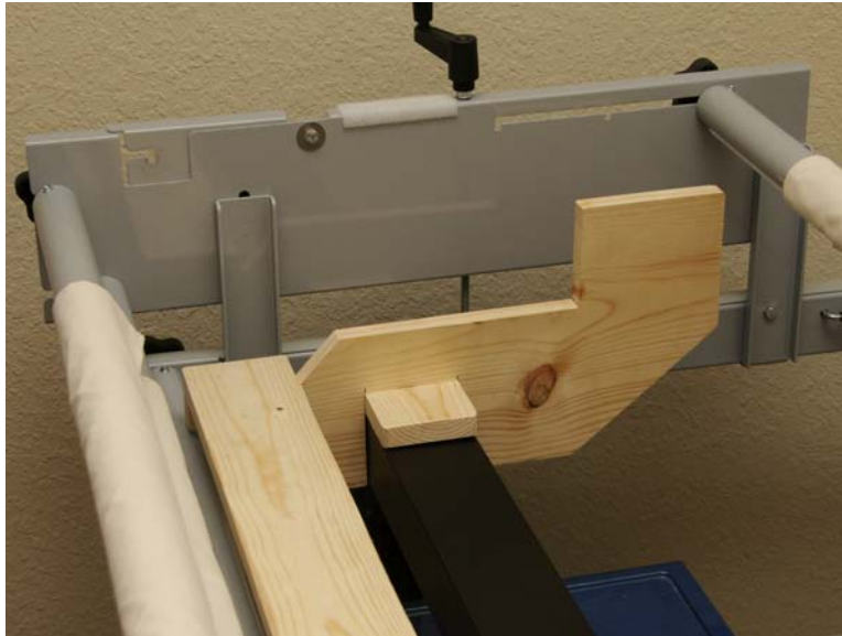
Figure 16. Shelf in position for pinning the top
