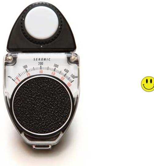
**Figure 21. Sekonic "Handi Lumi" model 246 illuminometer**
