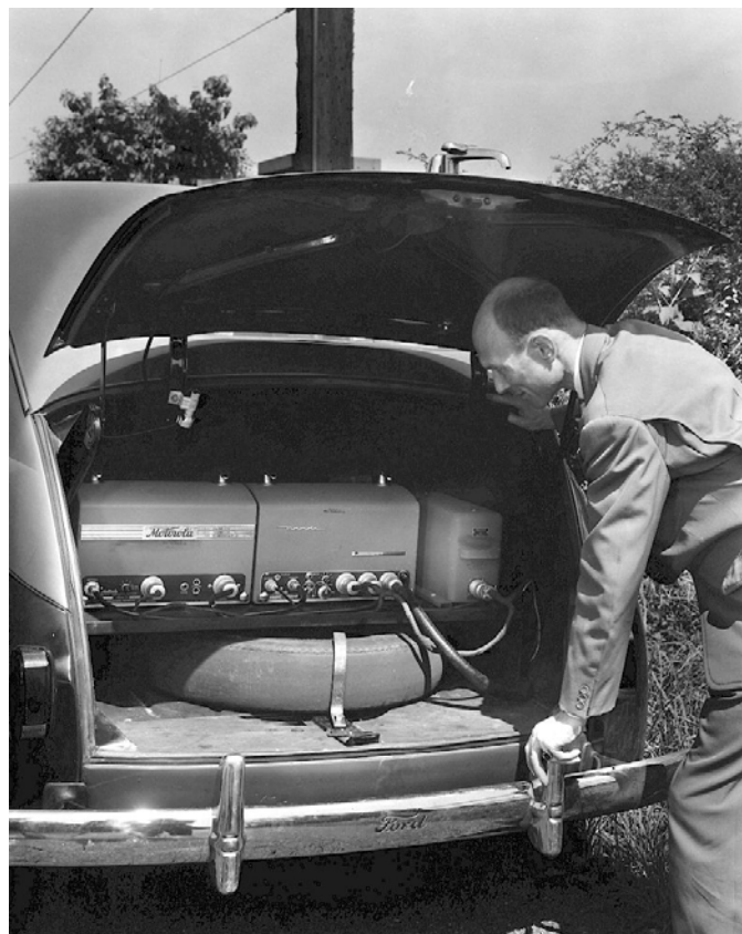
Figure 3. MTS station with Motorola receiver and transmitter
