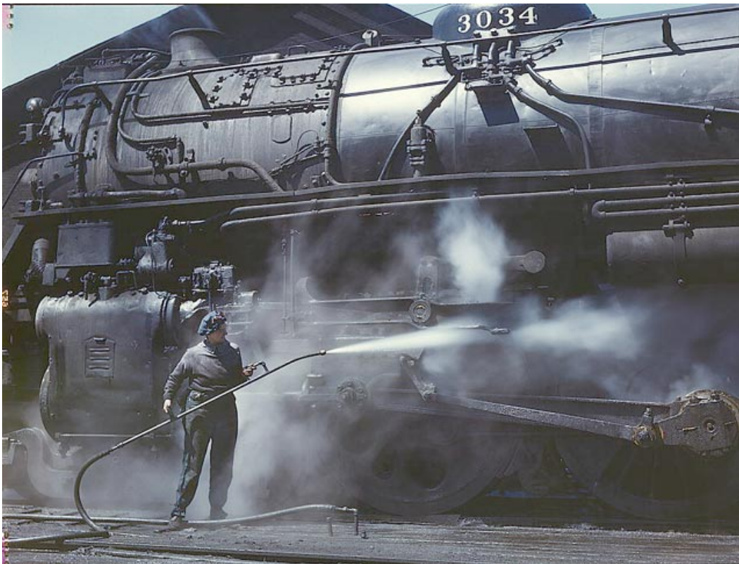
Figure 12. Steam cleaning a CNW class "H" locomotive
