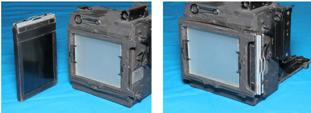
a. (r.) Back with no holder in place; (l.) Graphic-type film holder
