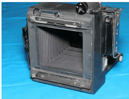
Figure 4. Graflok back with focusing plate removed
