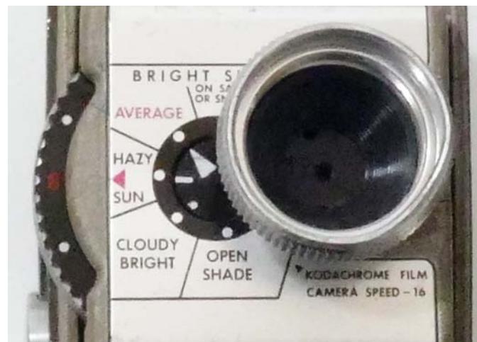
Figure 17. Kodak Medallion 8 movie camera aperture control
