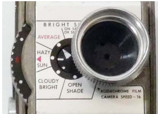
Figure 22. Kodak Medallion 8 movie camera aperture control
