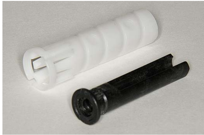
Figure 20. KwikPen control cylinder J and jackscrew driving cylinder H
