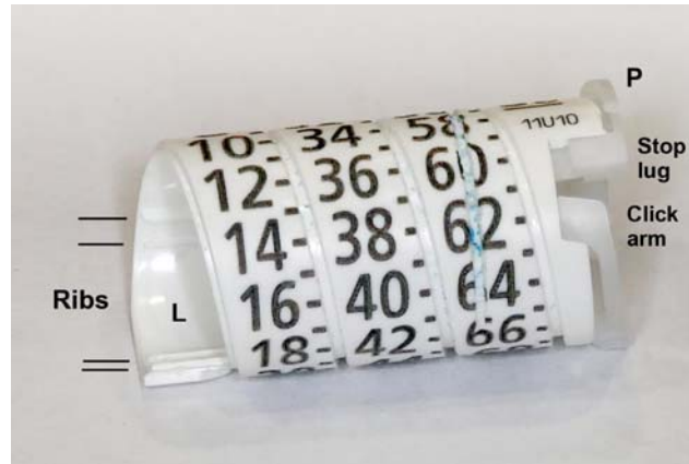
Figure 24. FlexTouch pen indicating cylinder, L and zero plate, P
