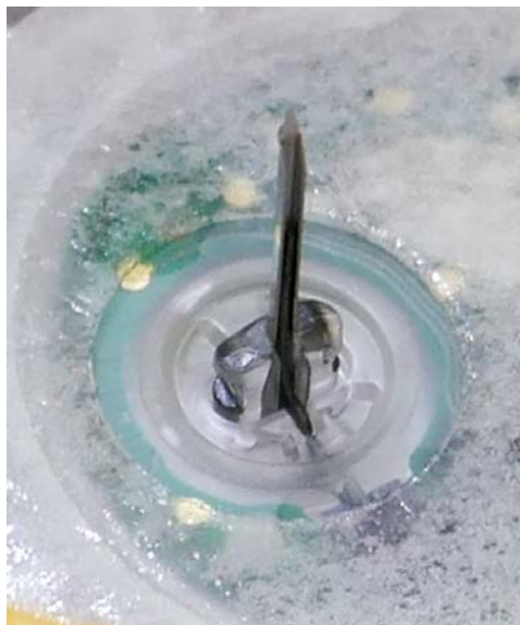
Figure 7. Probe in introducer needle
