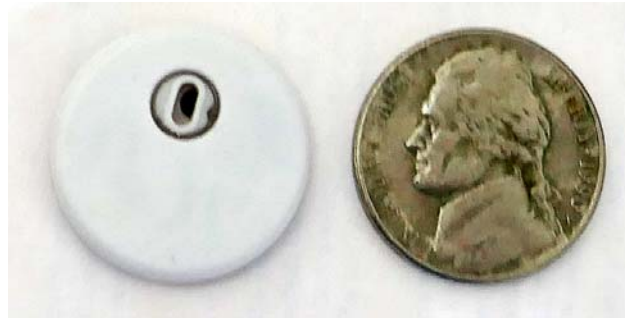
Figure 2. FreeStyle Libre 3+ sensor, from the back, with a nickel
