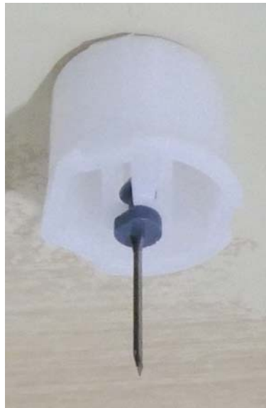
Figure 17. Introducer needle gripped by extraction plunger
