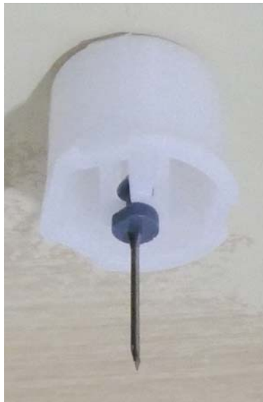
Figure 17. Introducer needle gripped by extraction plunger
