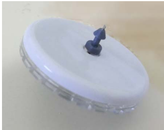
Figure 16. Sensor complete showing tail of introducer needle.
