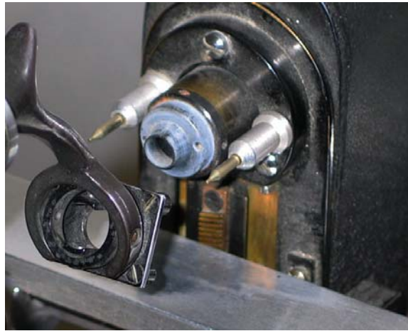
Figure 14. B&L Model 70 Vertometer—Reference axis locating pins
