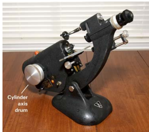
Figure 23. B&L Model 70—Cylinder axis drum
