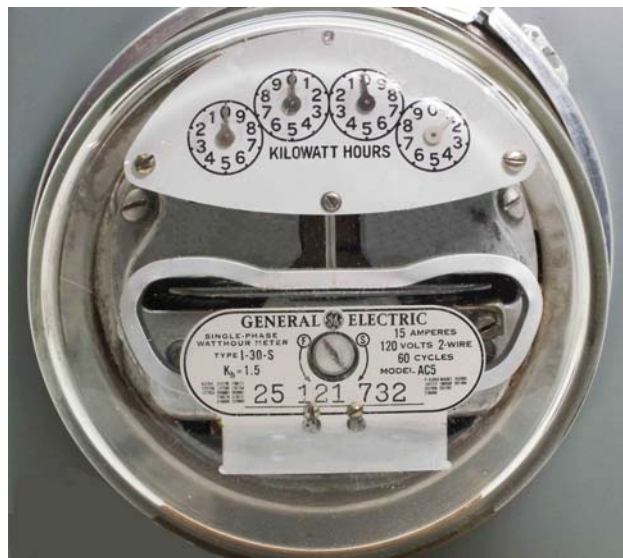
Figure 11. GE model AC5 watt-hour meter—“bowtie” magnet
