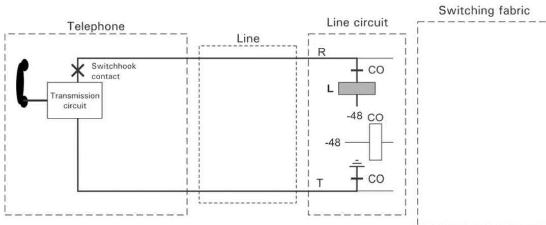
**Figure 4. Telephone taken off-hook**
