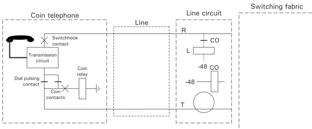
**Figure 12. Dial shunt contact**
