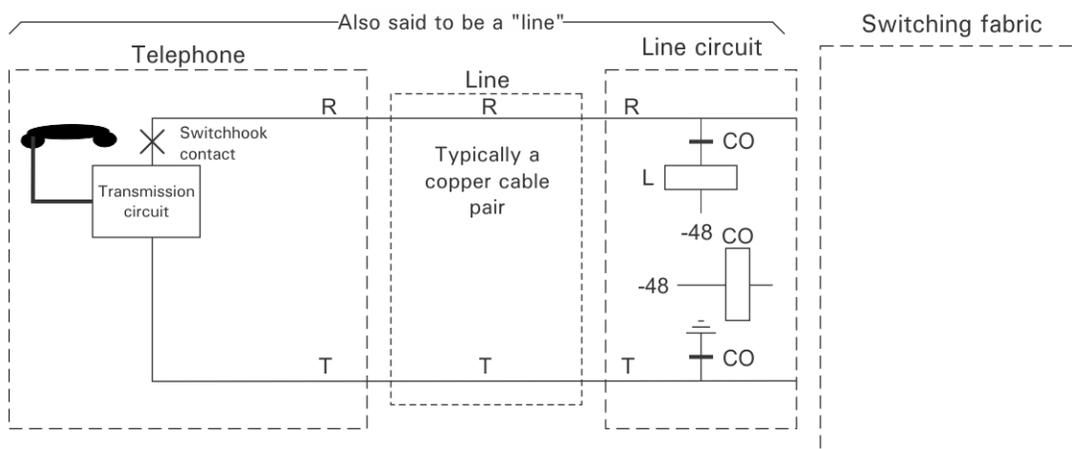
**Figure 3. Regular telephone line-idle**
