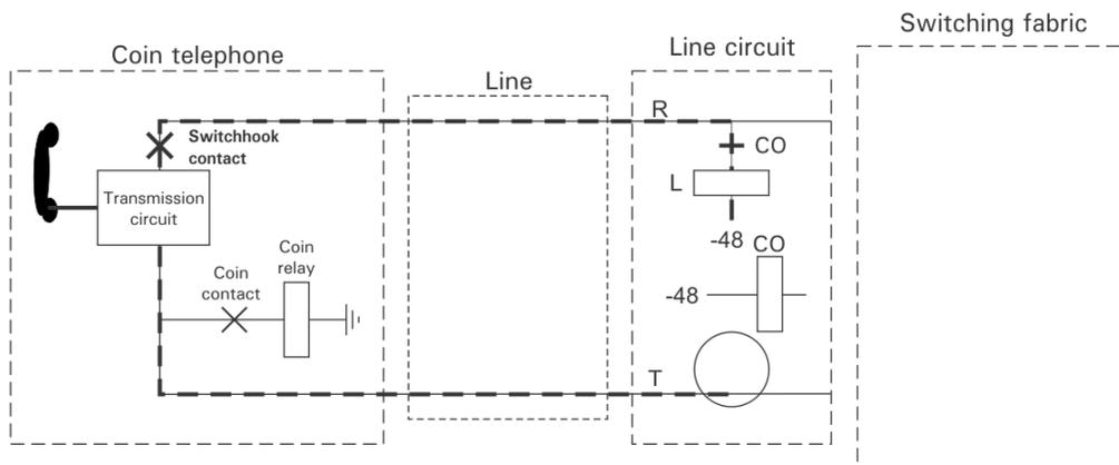
Figure 7. Coin telephone off-hook
