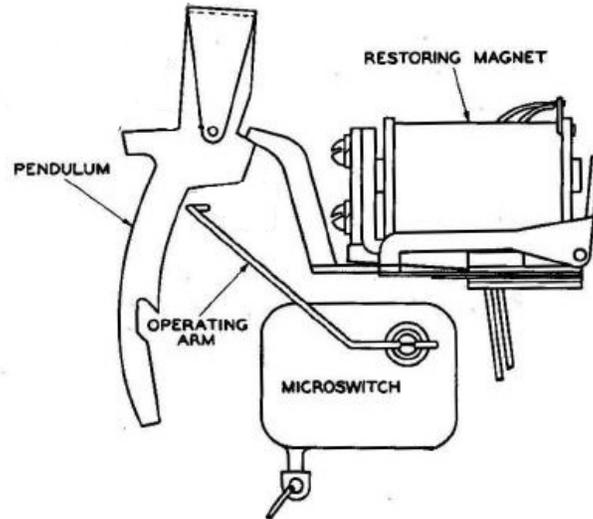
**Figure 24. Restoring magnet**
