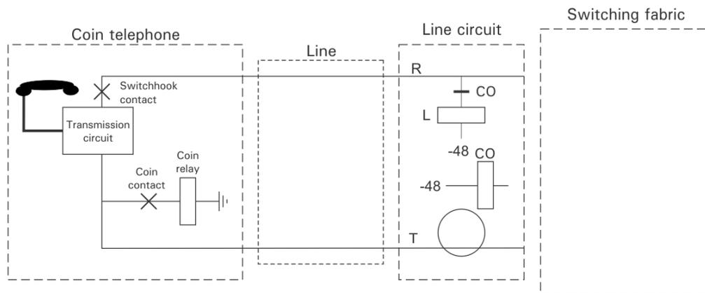
Figure 6. Coin telephone line–idle
