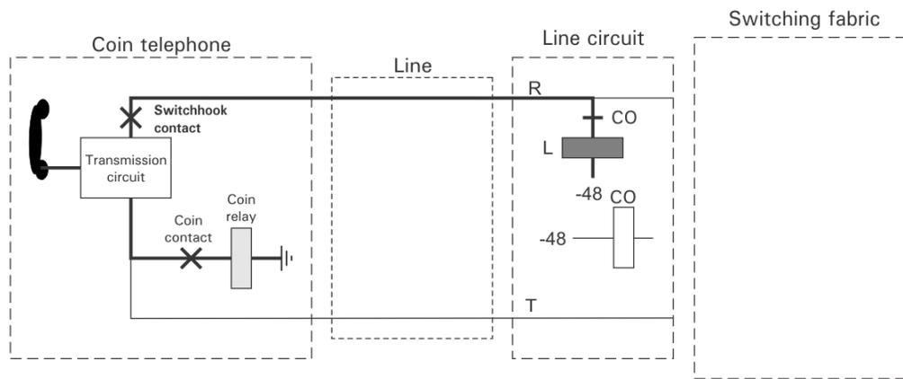
**Figure 8. Coin telephone off hook and coin deposited**
