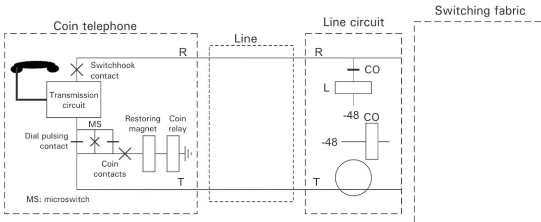
Figure 14. Automatic Electric two-nickel prepay coin telephone
