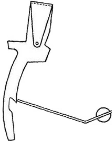
**Figure 16. Arm struck by nickel**
