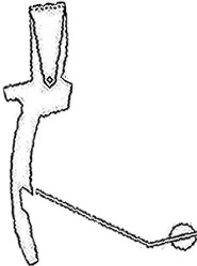
**Figure 22. Arm misses the tip of the notch**
