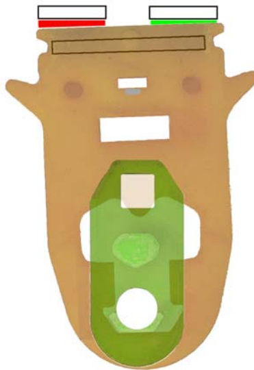
Figure 63. Relay energized, card moves down a little and swings
