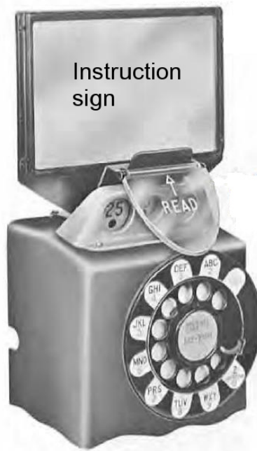
Figure 57. Gauge guard on postpay coin collector
