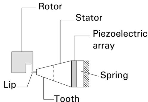
**Figure 4. Resilient lip on stator**
