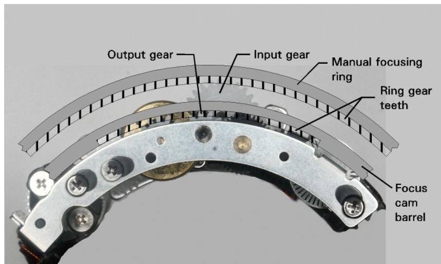
**Figure 13. Interface with manual focusing ring and focus cam barrel**
