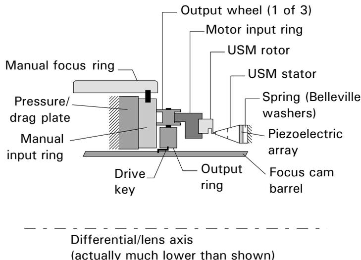
**Figure 10. EF lens—ring USM drive with mechanical FTM**
