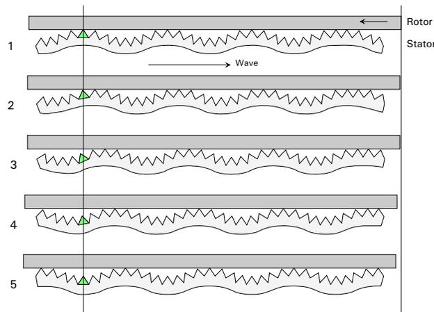
**Figure 2. Principle of ring USM motor**
