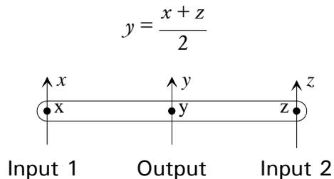
**Figure 5. Differential mechanism principle**
