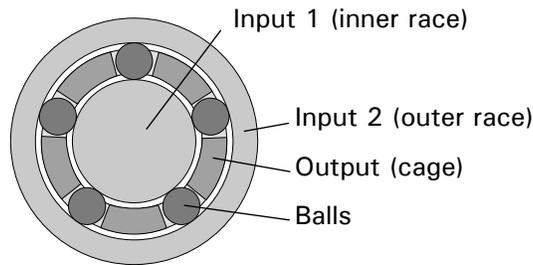
**Figure 14. "Ball bearing" differential**
