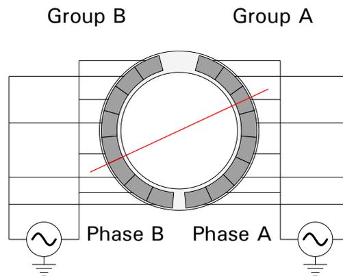
**Figure 1. Ring USM piezoelectric array**
