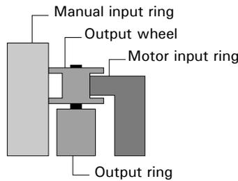
**Figure 9. Unequal-ratio differential**
