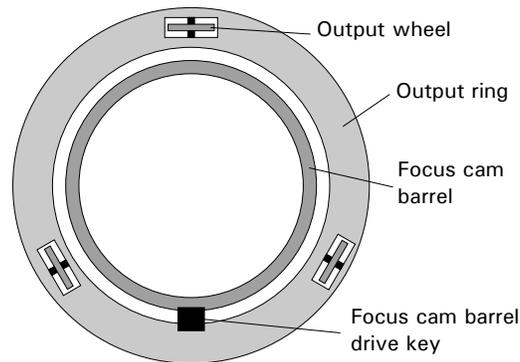
**Figure 7. Rotary wheel carrier differential—output ring**
