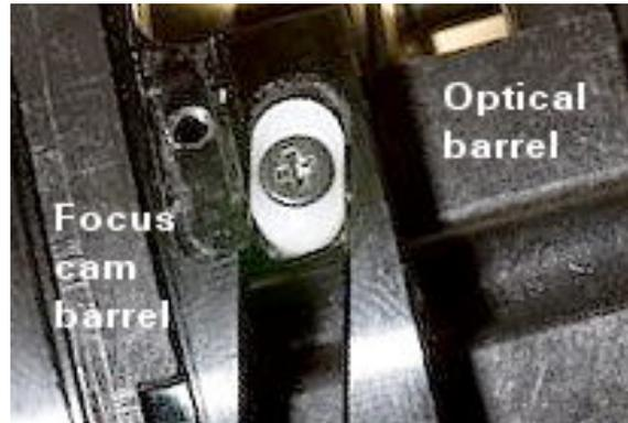
**Figure 16. Helical slot**
