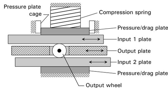
**Figure 6. Linear differential—wheel carrier type**
