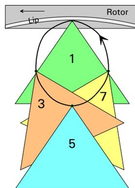
**Figure 3. Tooth tip motion**
