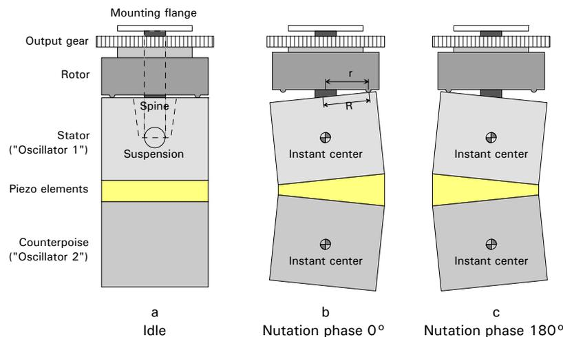
**Figure 11. Principle of the micro USM motor**
