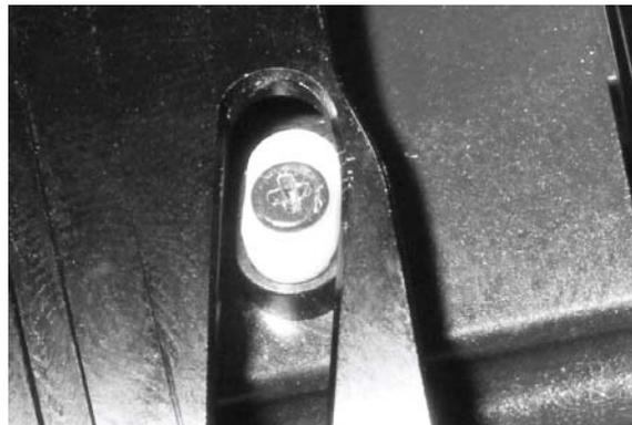
**Figure 17. Helical slot—distorted**
