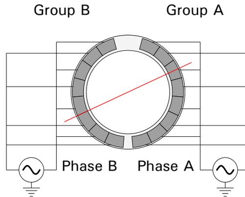
**Figure 18. Ring USM piezoelectric array**
