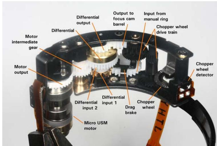
**Figure 12. EF 50mm f/1.4 USM drive assembly**
