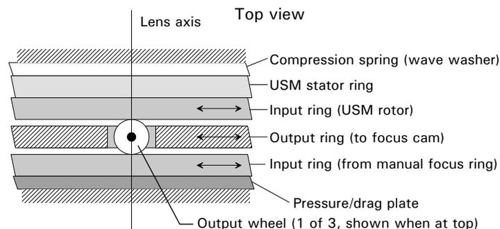
**Figure 8. Rotary wheel carrier differential**
