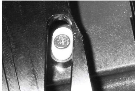
**Figure 17. Helical slot—distorted**
