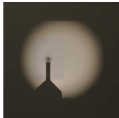
Rear sight in place Eye shift left 0.75 mm
