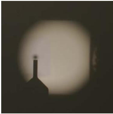
Rear sight in place Eye shift left 1.25 mm
