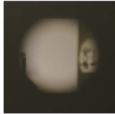
Rear sight in place Eye shift left 2.00 mm
