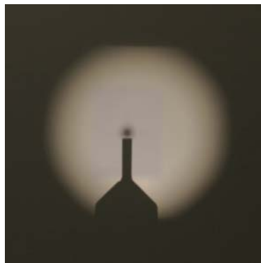
Rear sight in place Eye shift left 0.25 mm
