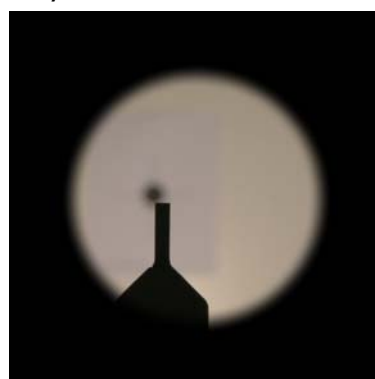
Rear sight out Eye shift left 0.75 mm
