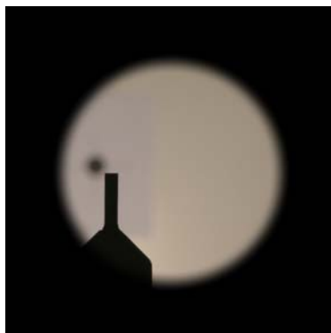
Rear sight out Eye shift left 1.50 mm
