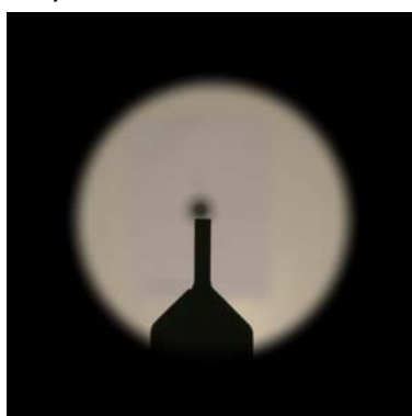
Rear sight out Eye shift left 0.25 mm
