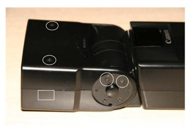
4. Remove the uppermost two screws (circled in the picture) from the pivot disk on each side. A 2mm Phillips driver is ideal.
