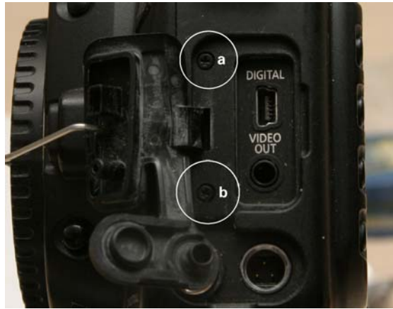
Figure 1. Removal of left cover (screws a, b)
