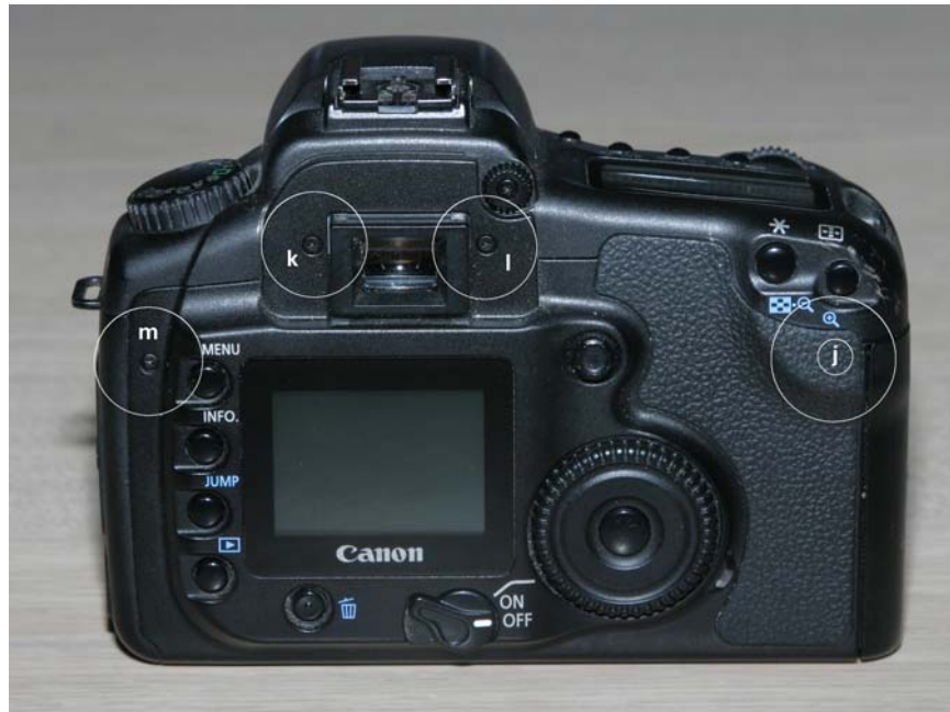
Figure 5. Removal of back cover (screws j, k, l, m)
