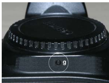
Figure 3. Removal of front cover (screw g)
