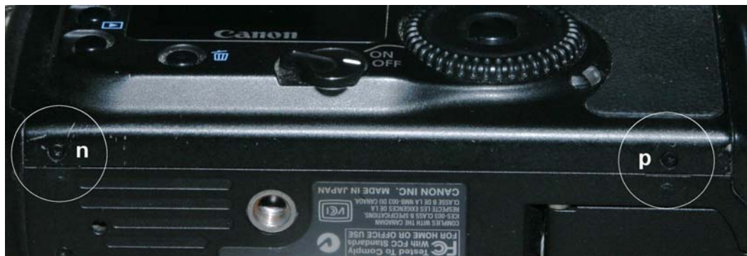
Figure 6. Removal of back cover (screws n, p)
