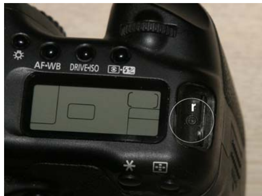
Figure 9. Removal of top cover (screw r)
